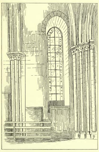
FIG. 2. LEANING WINDOW AND LEANING ENGAGED PILASTERS. LEFT AISLE OF NOTRE-DAME, NEAR THE ENTRANCE. ACCURATE DRAWING FROM THE SURVEY PHOTOGRAPH.
