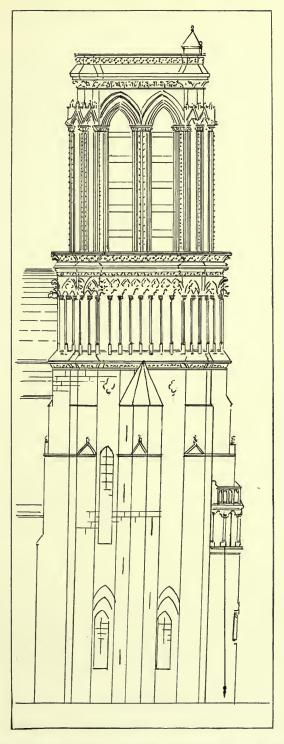
FIG. 3. VERTICAL BEND OF THE NORTH TOWER OF NOTRE-DAME. SLIGHTLY EXAGGERATED DRAWING. Compare with Fig. 6.
