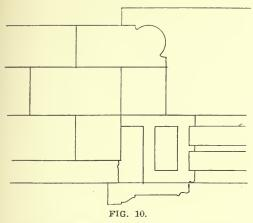
across the window from out to out of the brick casing and no more. It may or may not be worth while to make that 4-inch projection, to incur that added expense, for the sake of the slight additional space gained within. As to that, each separate case will
